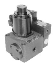
EFBG series proportional pressure and flow control valves adopt two electrical loops to control pressure and flow of hydraulic system respectively. Using very small pressure drop to track load pressure and control the pump pressure, it is an energy-saving valve.
